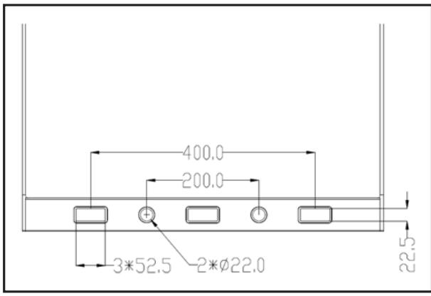
Use M20 screws with oversized washers to lock the bracket for installation. Screws are not provided in the package.
