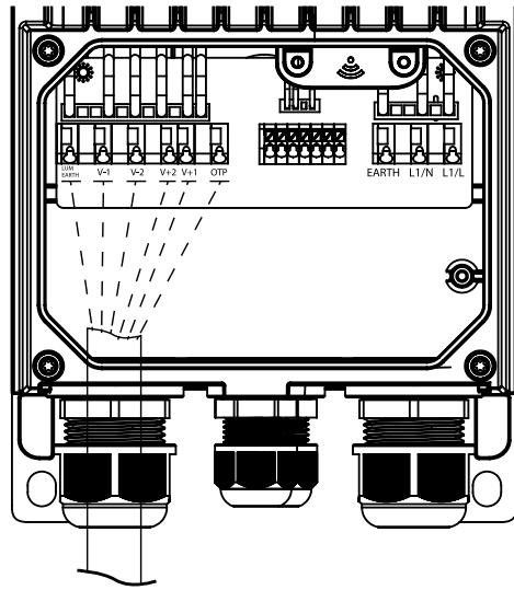
1200W lamps are directly connected to the **NFS-1200S210BC Inventronics Power Supply**. Note that the wire labels must correspond to the terminal position labels. After connecting the wires, use cable ties to tie the wires to the bracket to prevent the wires from moving around.
