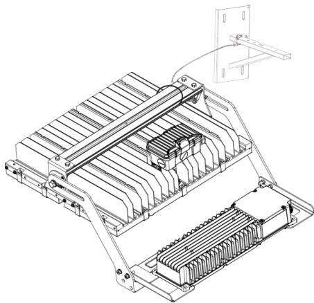
The safety cable is included with the luminaire and must be secured around the cross arm using the snap buckle, as illustrated. This cable serves as a fall-protection measure during maintenance or replacement. Important: It is not intended to bear the weight of the luminaire for extended periods and should not be used as the primary support.
